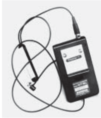
Image 16. A sensor allows each fanalet's position to be tracked in three-dimensional space.
